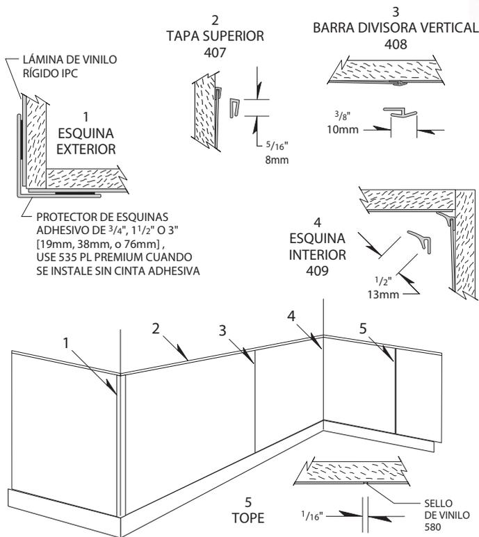
PARA UNA LÁMINA DE .080" [2mm], USE UNA TAPA SUPERIOR 417, UNA BARRA DIVISORA 418 Y UNA ESQUINA INTERIOR 419
