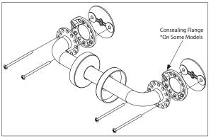
**Wing-Its Installation:** (Only compatible with the Vinyl Coated Grab Bars) 1. Using the flanges as a template, transfer the 2 holes per
