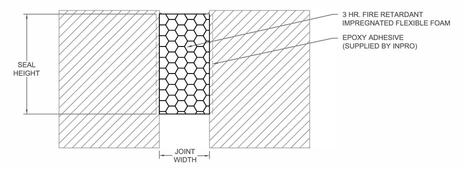
NOTE: SURROUNDING SUBSTRATE MUST MATCH OR EXCEED PERFORMANCE CAPABILITIES OF THE 990 FIRE RATED FOAM TO ACHIEVE FIRE RATING
