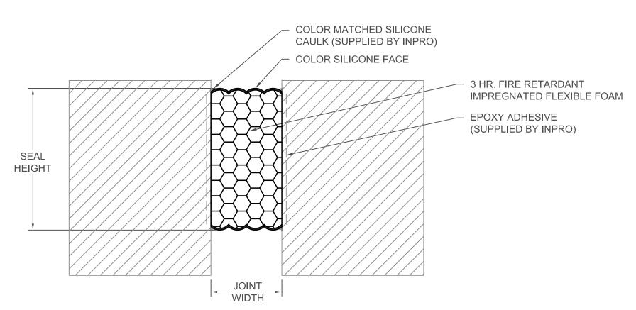
NOTE: SURROUNDING SUBSTRATE MUST MATCH OR EXCEED PERFORMANCE CAPABILITIES OF THE 990 FIRE RATED FOAM TO ACHIEVE FIRE RATING
