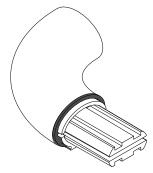
2. Attach Returns and Corners to retainer, leaving 1/16" [2mm] gap between Return/Corner and retainer allowing for adjustment. See Fig. 3. Note: Cut cover to length between the reveal pieces on the returns and/or corners.
