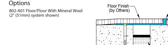
Flat Head Concrete Sleeve Anchor (7 per Frame @ 18" O.C.)
