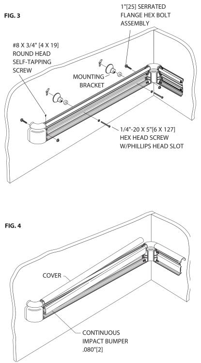
3. Using a 1/4" (6mm) drill bit, drill hole through the tab on the returns/corners for the top portion of the handrail Slide tabs onto top portion of retainer and fasten. For the lower portion of the handrail slip optional reveal onto returns/corners, slide tabs of returns/corners onto retainer and fasten. Loosely attach brackets to retainer. Mount on wall, level retainer and tighten screws to secure. See Figure 3.
