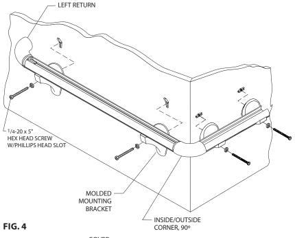
3. Position retainer against wall at desired height. Level and mark bracket holes on wall. Drill marked holes with 3/4" (19mm) drill bit for toggle bolts (drywall installation) or 1/2" (13mm) drill bit for lead anchor (concrete wall installation). Loosely attach mounting bolts to the brackets. Mount on wall, level retainer and tighten screws to secure. See Figure 3.
