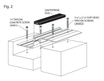
Install the architectural joint system on a level surface within the blockout. Make sure the top of the recessed frame is at a height level with the finished floor. This may require adding leveling compound to raise the top of the recessed frame.
