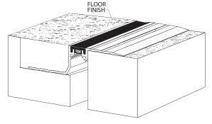
9. Insert the Santoprene seal into the recessed frame slot until the seal is flush with the tops of the frames.
